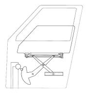
Figure 5: A power window simulation model
