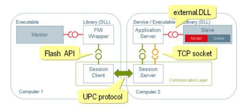
Figure 2: Implementation of FMI communication layer
