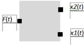
Figure 3.8: Port Mapping for Double Mass-Spring-Damper
