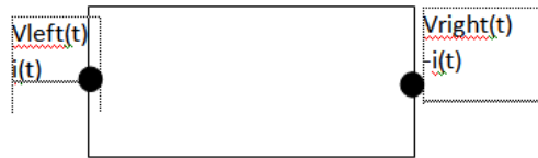
Figure 3.9: Resistor Port Mapping
