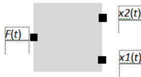
Figure 3.15: Port Mapping for Double Mass-Spring-Damper
