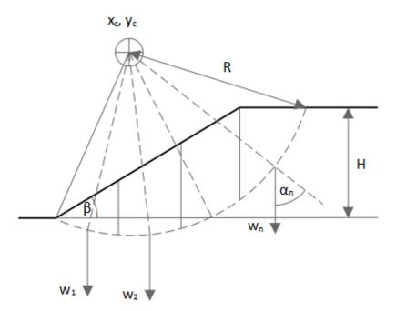
The applciation employs the Ordinary Method of Slices. Other methods of slope failure analysis, such as Bishop's Simplified Method, can be easily implemented.
