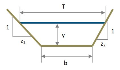
Given a trapezoidal channel, this application derives formulae for Sf and Fr. These are substituted into the differential equation, which is then numerically solved. Finally, the water surface profile along the channel is plotted.
