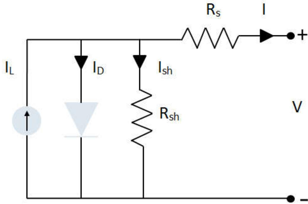
The behavior of a photovoltaic diode is often modeled with an equivalent circuit (illustrated above), and is described by the equation below.
