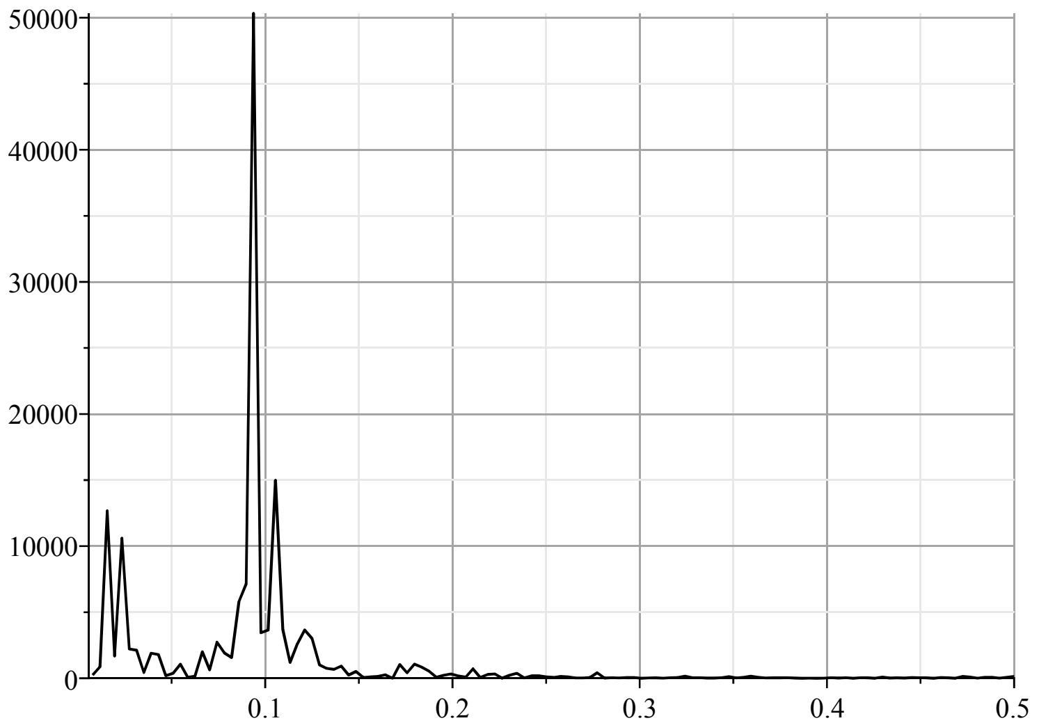
Note the peak at a frequency of  $0.09 \text{ years}^{-1}$ . Try zooming in and using the point probe to confirm the value of this peak frequency.
