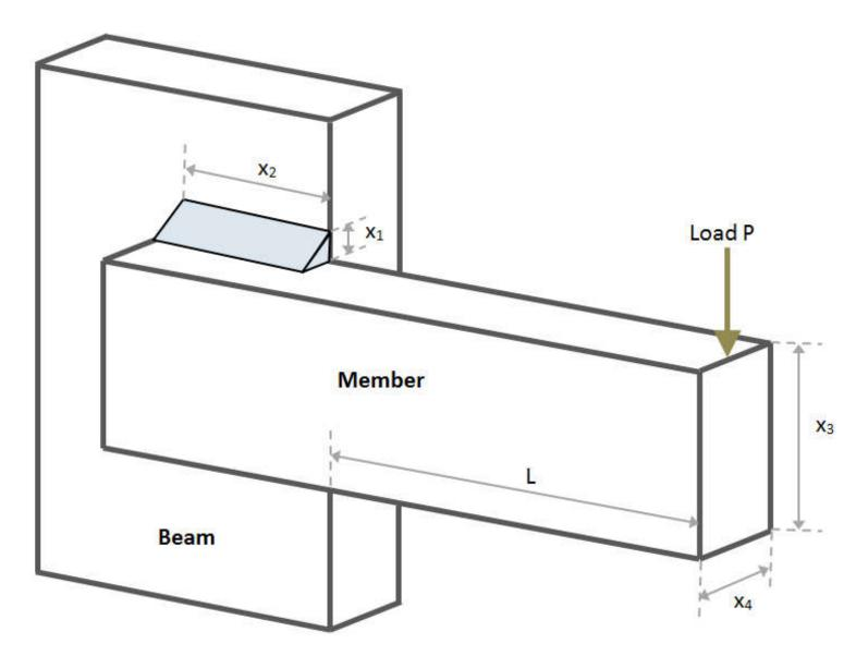
The total cost of production is equal to the labor costs (a function of the weld dimensions) plus the cost of the weld and beam material.
